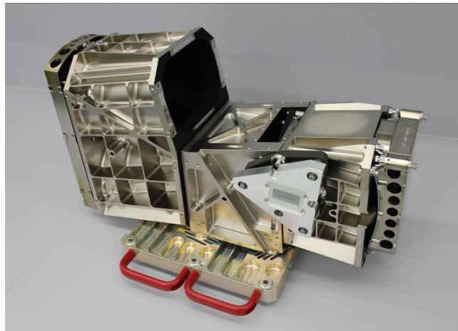
Figure 5. Optical system of the DESIS instrument, composed of aligned mirrors and housings. The light gray, triangular body is a detector dummy.
