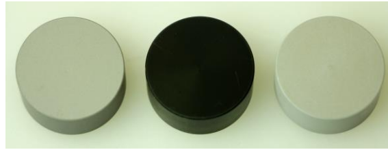
Figure 3. Different coated Al-42Si samples (f.l.t.r. black anodization, Acktar Fractal Black™ and plasma chemical coating).
